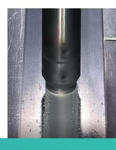
H2020 RESURGAM Project: 13 partners from EU including GISBIR are researching to apply Friction Stir Welding (FSW) to steel for panel asseblies and underwater robotic welding. FSW has low energy consumption and there is no need to use consumable materials.
